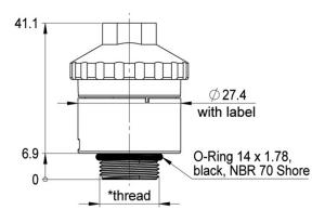
[\* thread is compatible with DIN 13 M16x1 and UNEF 5/8-24]
